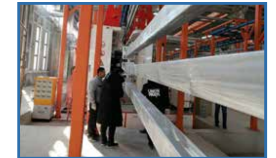
Automatic lift system for loading and unloading Buff zone for workpiece storage and cooling Fast and low chain speed transfer automatically Workpiece scanning system.
