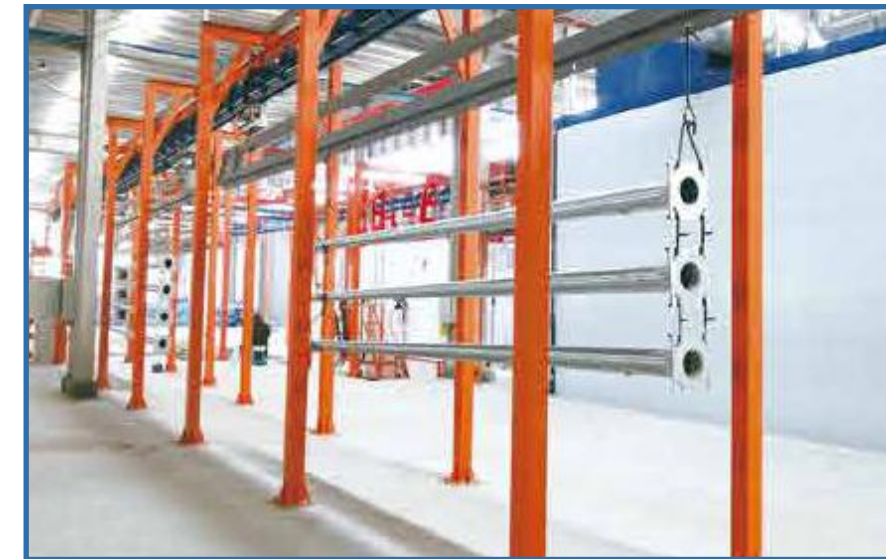
Automatic lift system for loading and unloading Buff zone for workpiece storage and cooling Fast and low chain speed transfer automatically Workpiece scanning system.
